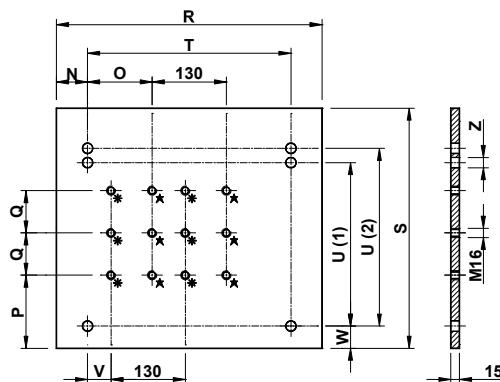
BM-T 70 支撑电机底盘 (已包括) / Motor supporting baseplate for BM-T 70:
