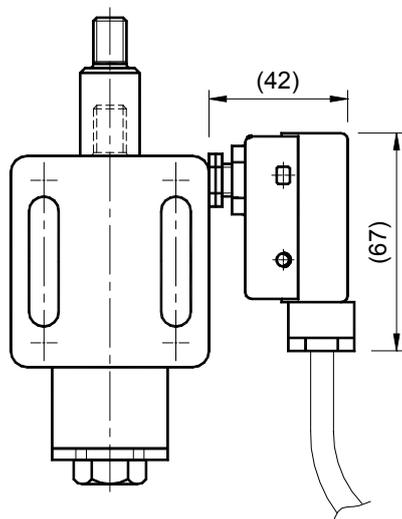
*The elastic spring elements TEN BLOC can be supplied, on demand, with travel-end switch "E". The applications with FCE are various, since they allow to check and to prove the correct functioning of the machine, but also to receive or to give control signals for the carrying out of the mechanical functions. This system is particularly useful when you want to grant the integrity of the machine and/or where the workers' safety must be protected.*
